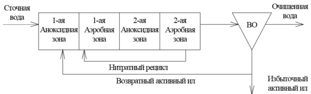
Fig. 4.23. Circuit diagram of the Bardenpho process
