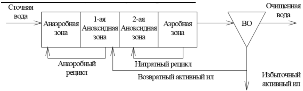
Fig. 4.22. Schematic diagram of the Modified UCT process
