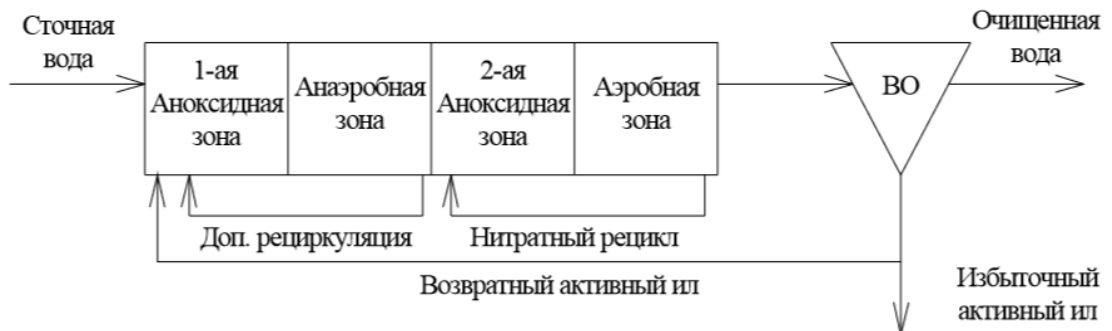
Fig. 4.26. Schematic Diagram of the Modified JHB Process
