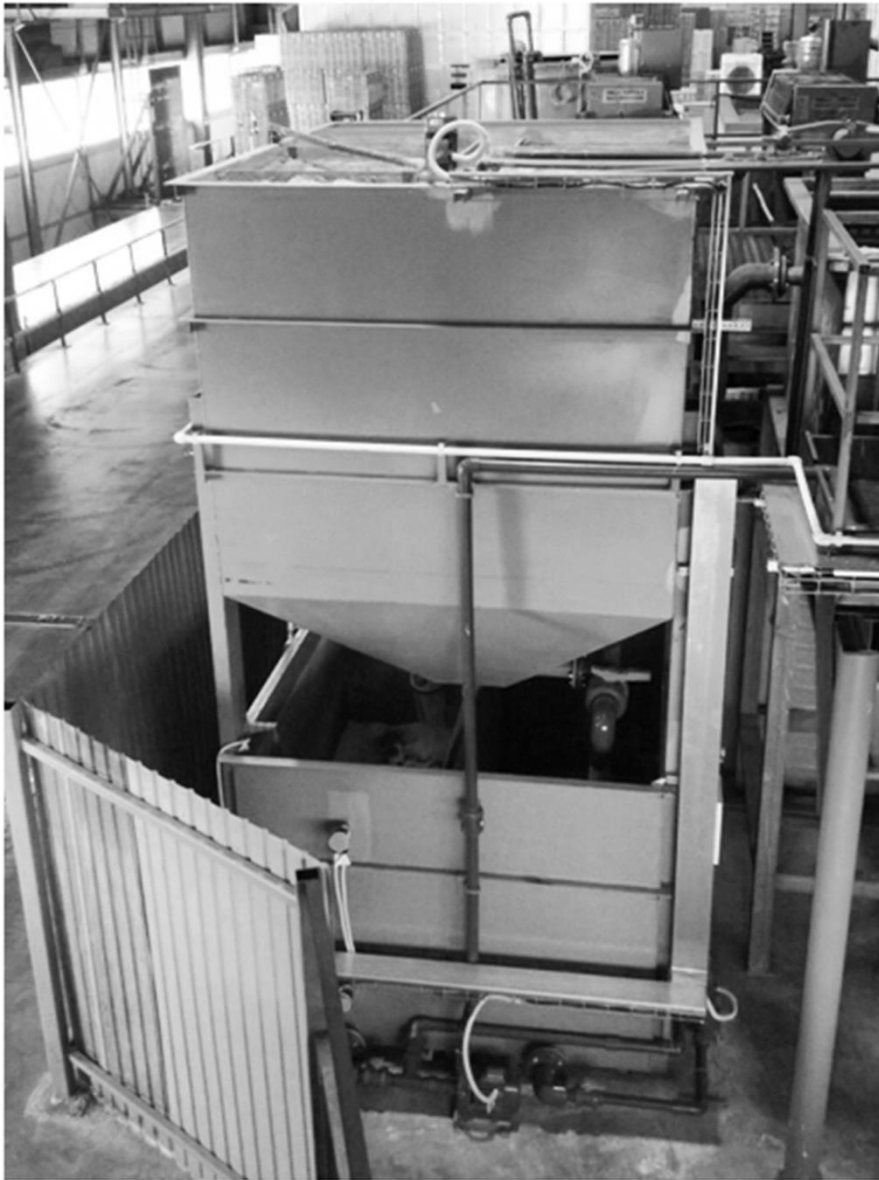
Fig. 4.31 - Photo of the sweep of the shell sample of the flotation tank
